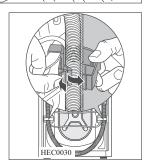
**3.** Unscrew the three bolts with the supplied spanner
